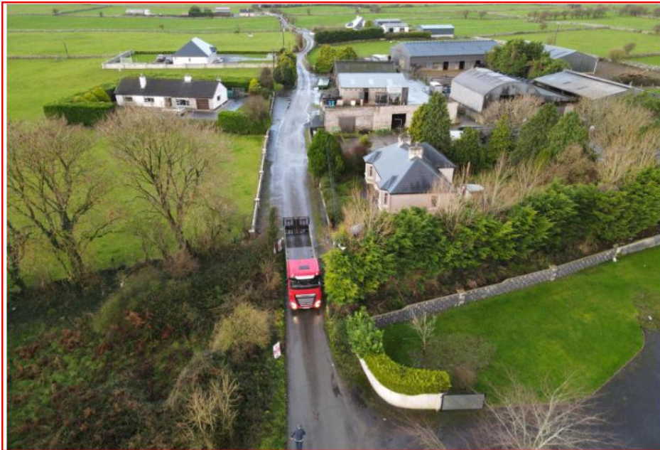
Inadequate width at N83 junction determines queuing on the N83 to turn right.
