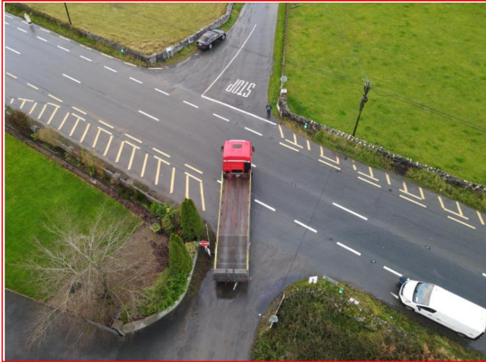
Note that absence of kerb radii determines that HGV turning movement has to cross lane to contraflow lane to turn left.
